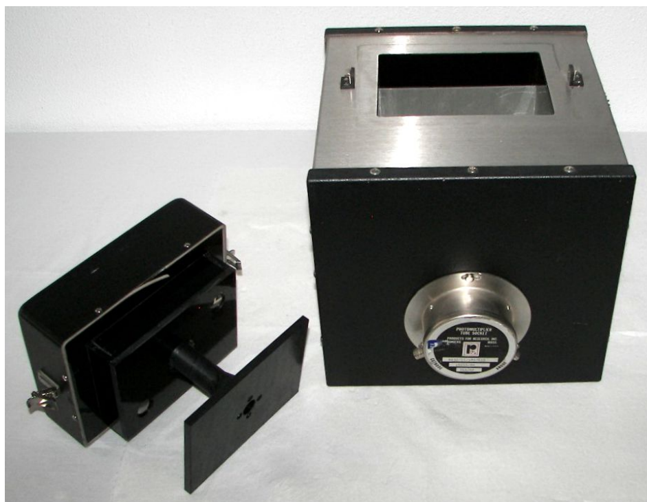
Figure 3 – Dry ice-cooled PMT housing model TE-241 manufactured by Products for Research. The dry ice chamber is shown open. This housing accommodates standard 53.4 mm diameter end-on PMTs.
